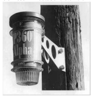
Bowden Bros. introduce the Pathfinder 360 Alpha, a sophisticated overhead line fault passage indicator that will detect earth faults and phase to phase faults of either a permanent or a transient nature, and indicate with both a high intensity Xenon Gas flashing light and a bright LED. For remote communications functionality see PATHFINDER 360 ALPHA GSM
